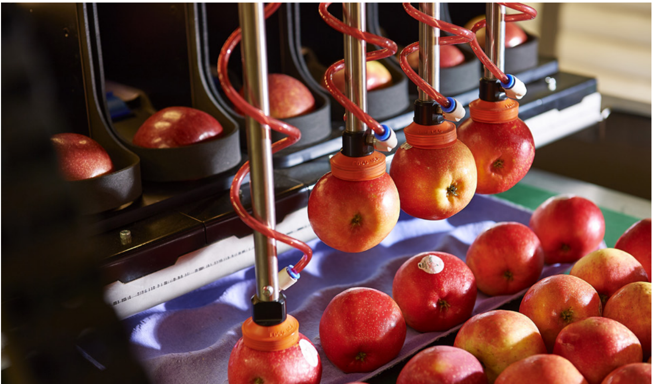
A Robotics Plus apple packer packs at twice the speed of a human, all day, everyday. Image supplied by: Robotics Plus
